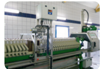
Automatic cake discharge boom
