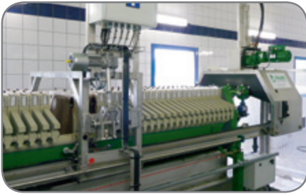
Automatic cake discharge boom
